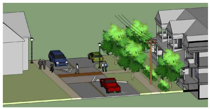
Axonometric View of Sidewalk 'Bump-Out' and raised crosswalk.
