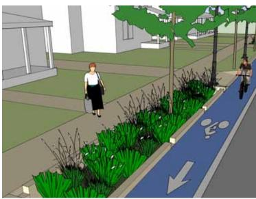
Innovative stormwater treatment options can be incorporated into new development.
